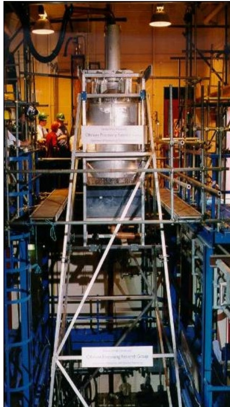
Figure 11 Pilot scale bundle for motion tests
